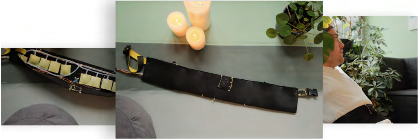
Figure 1: Zen Belt - Hardware Prototype for Guided Breathing Exercises
