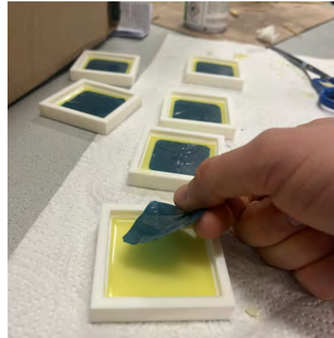
Figure 6: Production of the final version of the silicone pads
